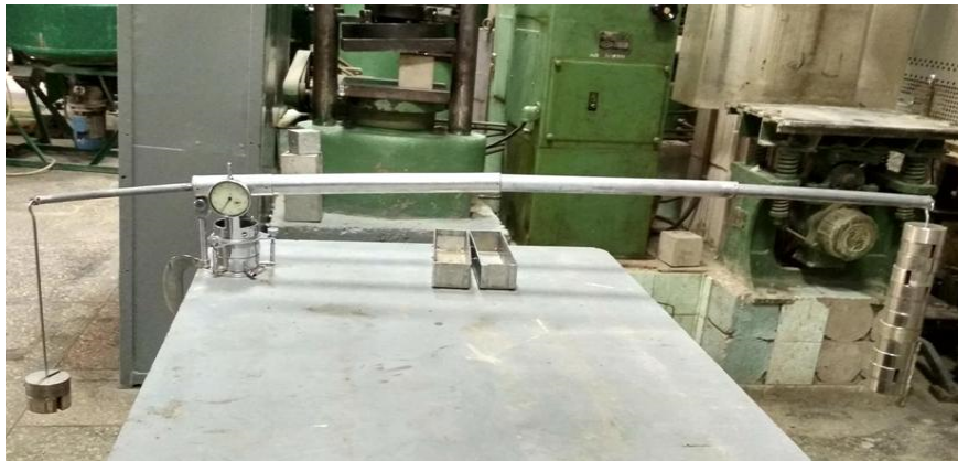
Figure 2. Tests on the soil samples with the method of virgin compression.
