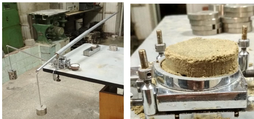
Figure 1. Tests on soil samples with the method of direct shear.
