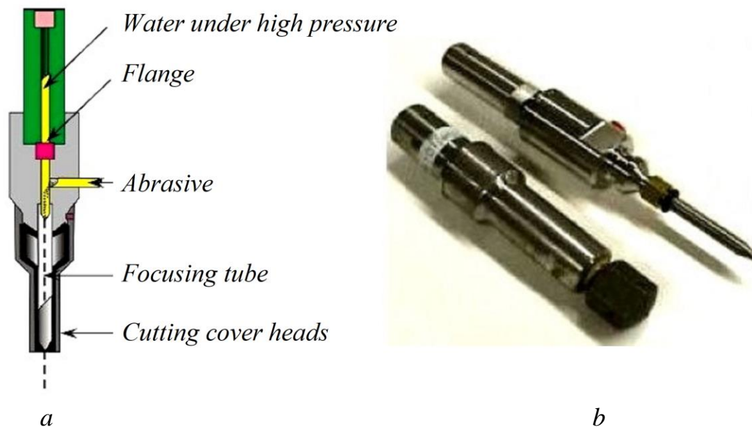
Figure 4.7 – Diagram (a) and photo (b) of the cutting head for AWJ
