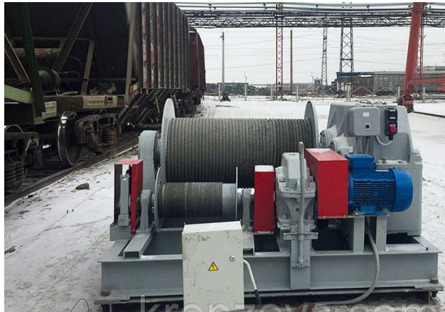
Figure 3. Shunting sheave-type winch.
