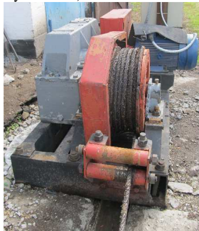
Figure 4. Capstan shunting winch.
