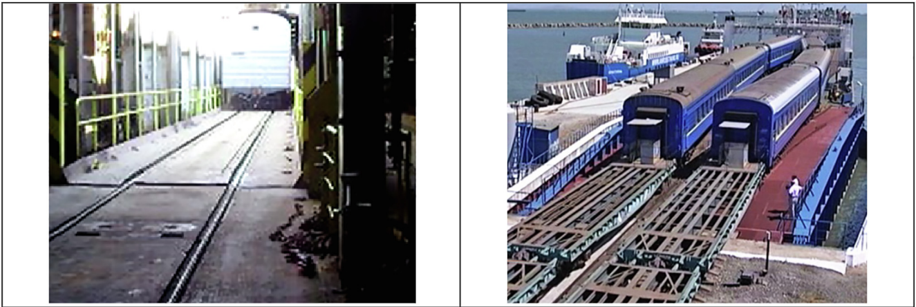
Fig. 2. Loading of passenger cars on a train ferry over the loading ramp.
