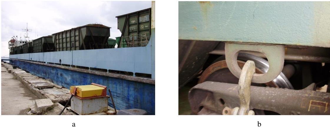
Fig. 1 Hopper cars transported by a sea vessel: a – rail cars on the sea vessel; b – attaching the hook to the towing shackle
