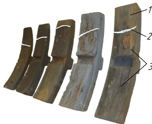
Figure 1. Appearance of brake pads which became unsuitable for further use due to the dual wear, but still with large remaining intact part of the working body: 1 – upper adverse wear; 2 – division line of wear areas; 3 – intact brake friction area of the pad reduced to the value of the upper wear
