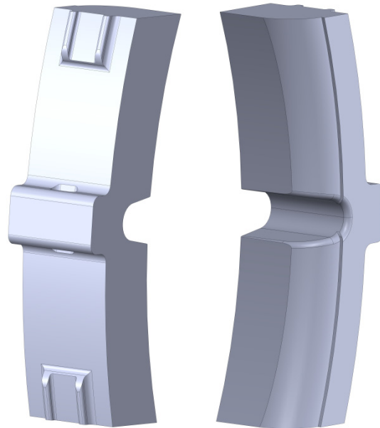
Figure 12. Spatial model of the composite brake pad.
