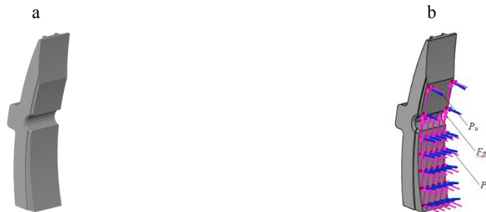
Fig. 3. Spatial model of the brake pad (a) with excessive wear (b) design diagram of the pad.
