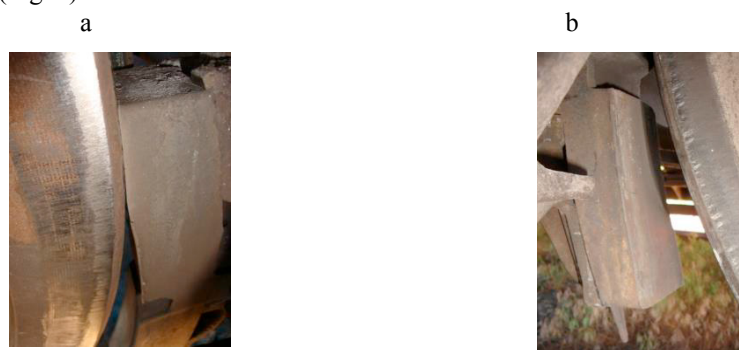
Fig. 1. Dual wedge-shaped wear of a brake pad (a) upper edge of the pad leaning against the wheel (b) abnormal gap between the wheel and the lower edge of the pad.
