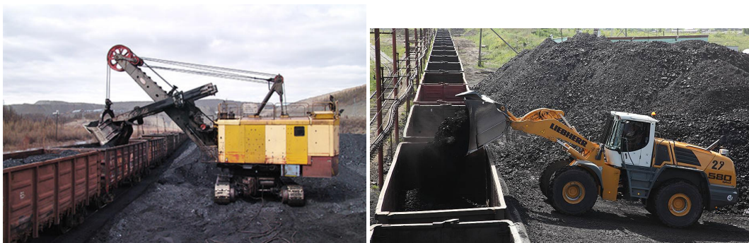
Figure 5. Loading of gondola cars with bulk cargo using loading devices of intermittent operation.
