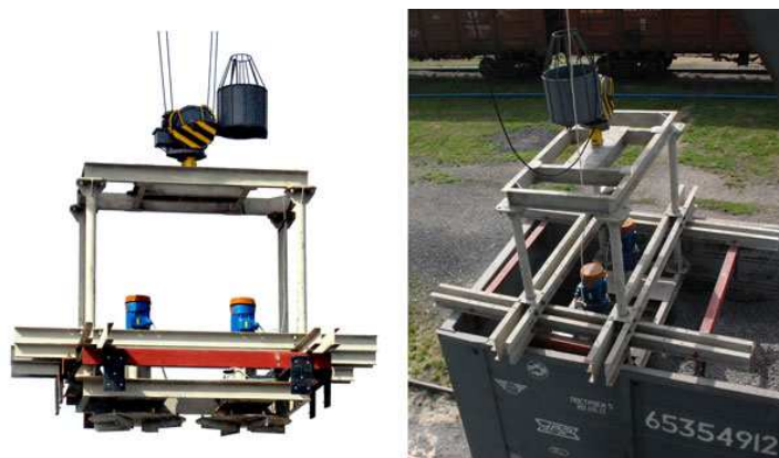
Figure 7. Leveler attachment for bulk cargo in gondola cars.
