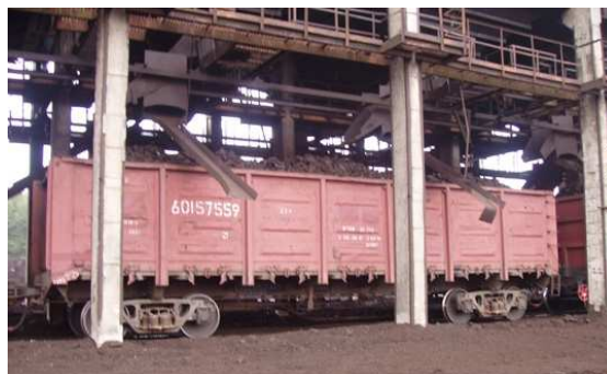
Figure 3. Loading of gondola cars with bulk cargo using a continuous loading device.
