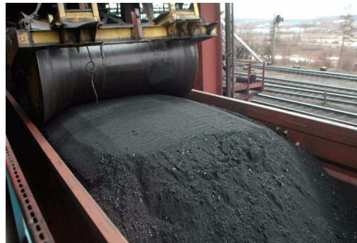
Figure 4. Compaction of the bulk cargo surface in the gondola car body.
