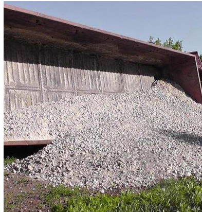
Figure 1. Consequences of rollover of a gondola car with bulk cargo.
