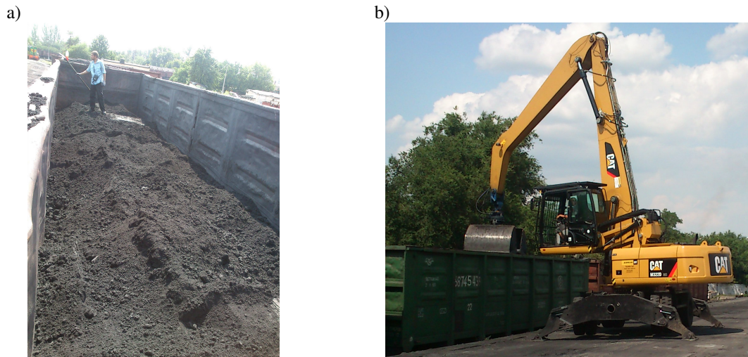
Figure 6. Common methods of levelling the bulk load: a - manually; b – with a clamshell excavator.
