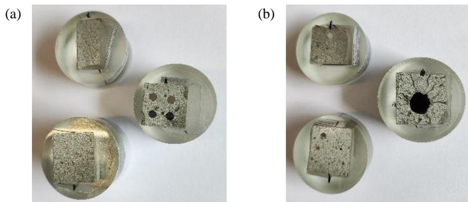
**Figure 4.** Specimens prepared for nanoindentation: (a) – from models with steel wire reinforcement; (b) – from models with composite reinforcement
