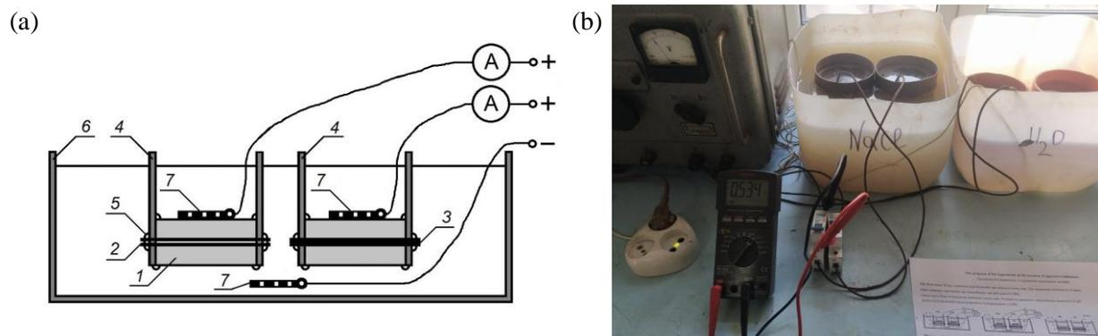
**Figure 3.** Experimental installation with sleeper models with steel wire and composite reinforcement for the study of electro-corrosion processes: *a* – schematic diagram; *b* - general view
