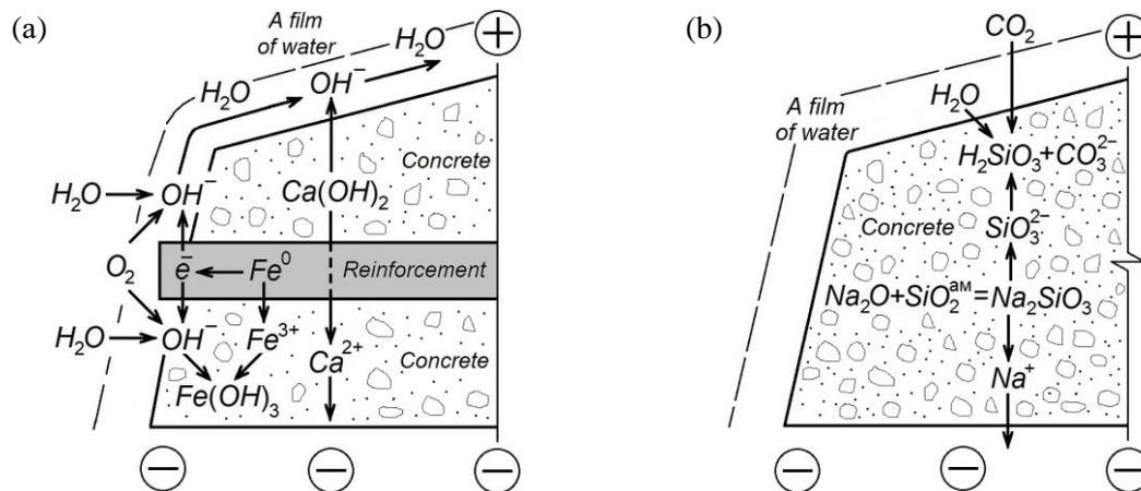
**Figure 2.** Diagram of current flowing through concrete and steel reinforcement of sleepers and corrosion processes [1]: (a) – current flowing through concrete and reinforcement and electro-corrosion of reinforcement; (b) – intensified corrosion of concrete due to ASR
