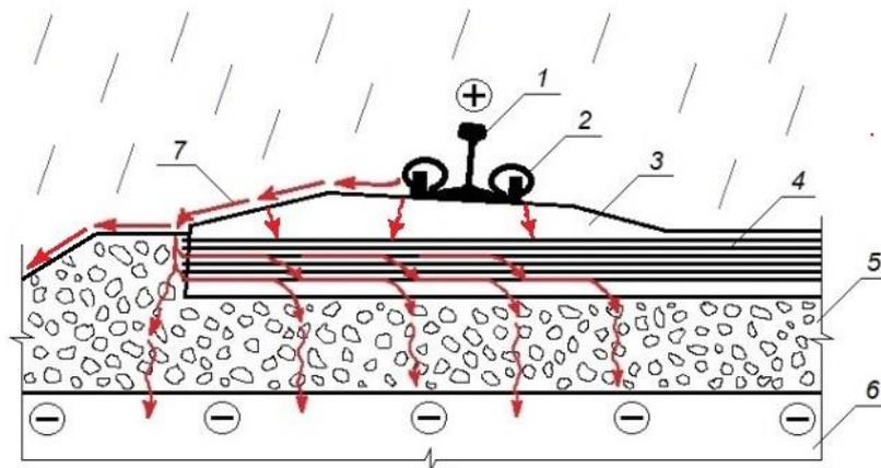
**Figure 1.** Diagram of leakage current flowing through sleeper and ballast in wet weather [1]: 1 – rail; 2 – rail fastener; 3 – concrete of the sleeper; 4 – reinforcement wire; 5 – ballast; 6 – roadbed; 7 – leakage current
