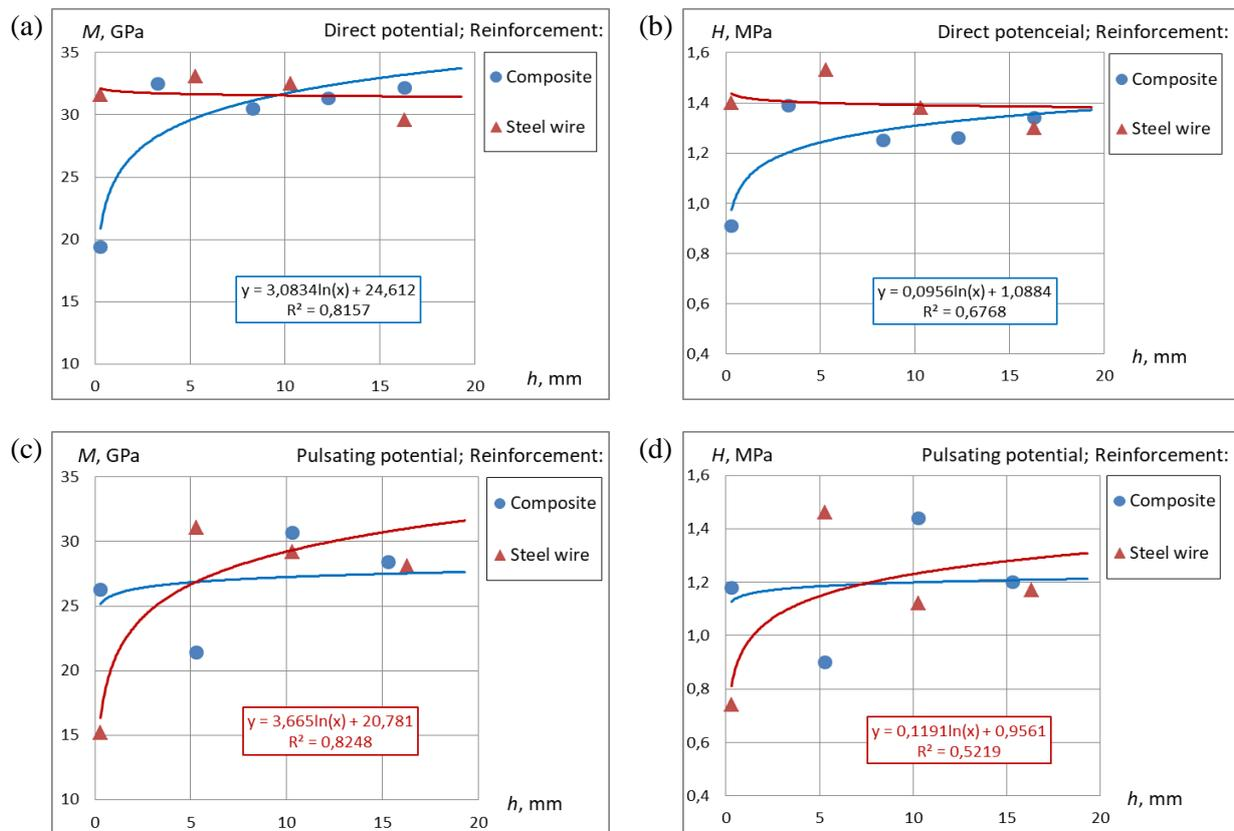
**Figure 6.** The dependence of the elasticity modulus  $M$  (a, c) and the hardness  $H$  (b, d) of cement paste on the distance  $h$  from the bottom face (negative potential) according to the results of nanoindentation after exposure to direct potential (a, b) and pulsating unidirectional potential (c, d)
