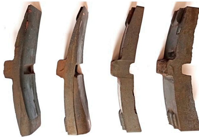
Figure 1. Composite brake pads unusable for wagons.
